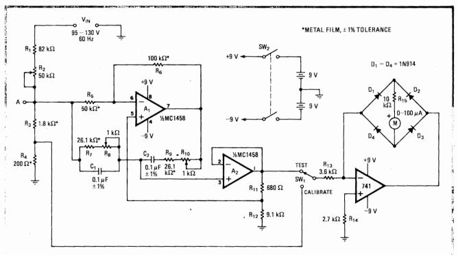
Handling harmonics. Wien-bridge notch filter rejects 60-Hz power-line fundamental frequency so that total harmonic distortion present in signal can be measured. Meter measures THD over 0-to-10% range. An rms-responding meter should be used, but an average-responding meter is acceptable. Results are displayed in percent, with an accuracy directly proportional to the tolerance of resistors in divider R<sub>3</sub>-R<sub>4</sub>.
